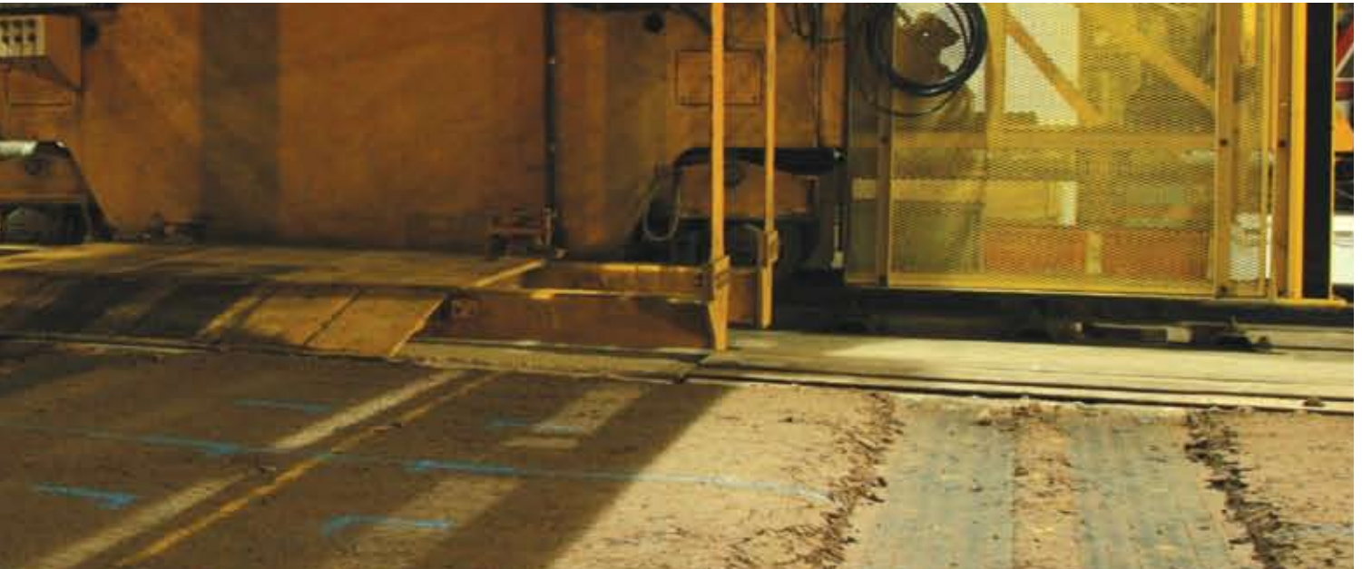
Trafficking trials by TRL proved the performance benefits of the TriAx geogrid compared with Tensar biaxial geogrids.
